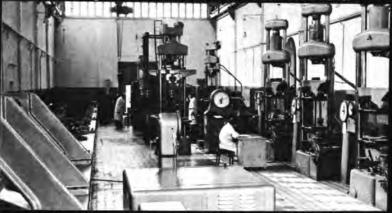
Laboratory workers test dust control methods.
