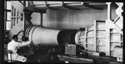
The wind tunnel at the Institute of Mine Safety. Checking elevators under simulated mine conditions.
