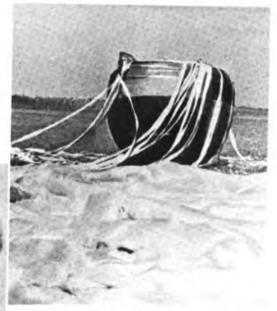
Tests of soft landing of a research station
