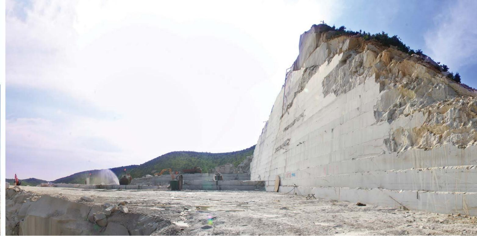
The Aeguk Stone Dressing Plant located in Yonha-dong, Haeju, South Hwanghae Province, is famous for quarrying granite which conforms to all the qualitative requirements for the building stone at a higher level. Its annual quarrying capacity is tens of thousands of cubic metres.
