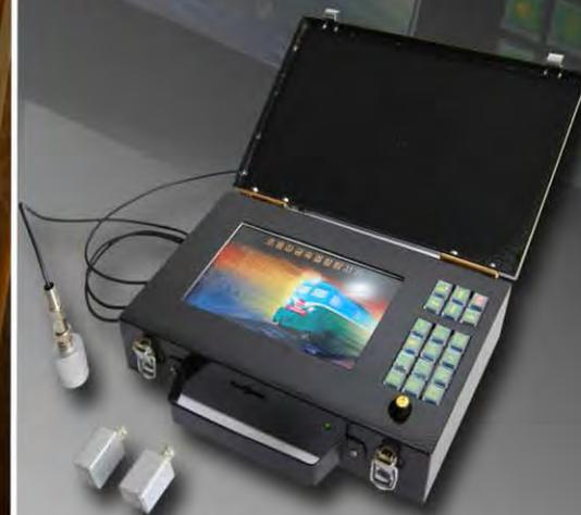
With a transmitter that can monitor the depths of over 5 000mm in the axle to detect cracks and a receiver that can amplify the signal up to 80 dB, it can continue detecting for over 8 hours through minimized power consumption as suited to its portable character.
