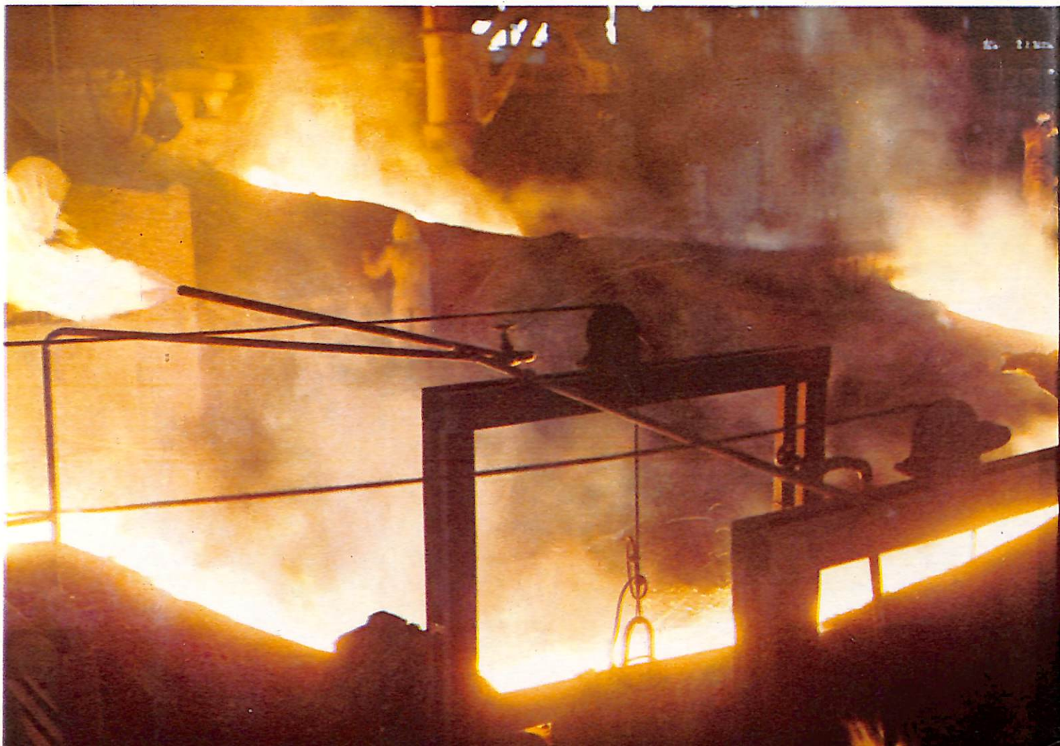
Molten iron being tapped from the new blast furnace No. 7.
