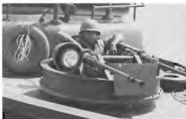
The PBR carried heavy fire power for such a small boat. The forward turret carried a pair of .50 caliber machine guns and a co-axially mounted searchlight. Late in the war a 20mm cannon was fitted in the turret, replacing one of the flinties and was fired alongside the remaining flinty.
