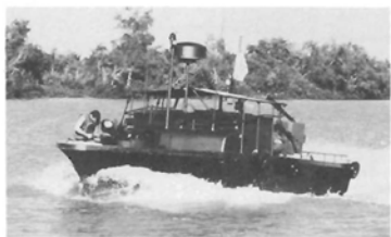
(Above) A PBR Mk II moves up a waterway in the Mekong Delta. The main visual difference between a Mk I and Mk II PBR was the curved portion of the superstructure on the Mk II. The round object atop the pole is a Raytheon 1900/W radar unit used for night patrols. (US Navy)
