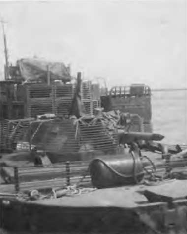
Another interesting modification was the replacing of the 40mm turret on this Monitor with the turret from an LVTH-6 Amtrac mounting a 105mm howitzer. Bar armor protection has been added around the turret. (Mesko)
