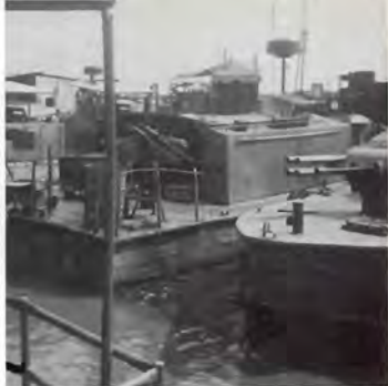
This ASPB has had the original single machine gun mount replaced by a twin mount. Note how the guns can receive ammunition from both sides. Unfortunately while the twin .50 caliber machnegun mount gave the Vietnamese a tremendous amount of firepower its range often led to civilian casualties outside the immediate battle area which did little to endear the Vietnamese Navy to local inhabitants. (Mesko)
