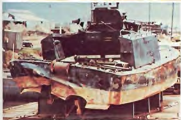
Mines were a constant problem for the riverine forces. This Assault Support Patrol Boat (ASPB) shows just how deadly a mine could be. The mine detonated under the boat's stern, killing or seriously wounding the entire crew. (Beneditti)
