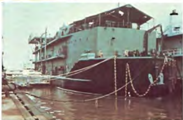
A non-propelled barracks ship at Vung Tau. These barracks ships provided much needed berthing facilities for Mobile Riverine Force personnel but had to be towed from area to area which caused serious mobility problems for the force. (Mesko)
