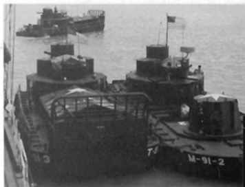
The differences between an ATC and Monitor can be seen here. The most evident difference is the spoon bow of the Monitor mounting a 40mm turret. (US Navy)
