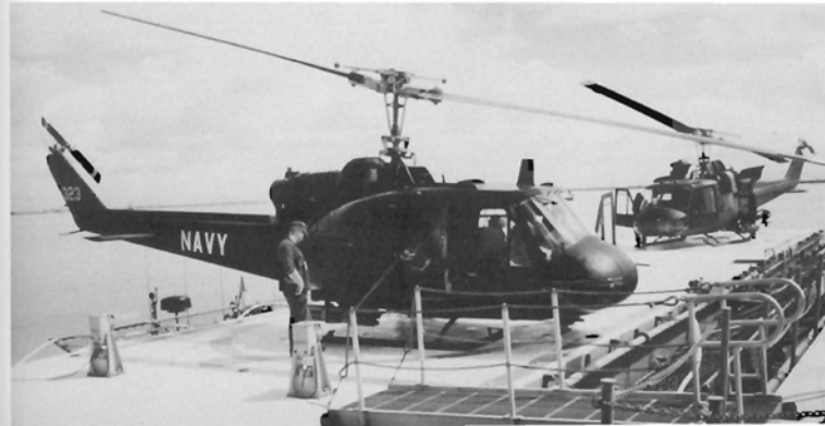
A detachment of two Hueys operated from this barge at Nha Be. The nearest UH-1 has a .50 caliber machinegun mounted in the starboard door gunner's position. (US Navy)
