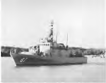
On patrol USS Ready (PG 87) is one of the new fast patrol gunboats designed for blockade and surveillance. However, its large size and shallow draft allowed longer patrols, heavier weapons and the ability to operate very close to the shore in order to provide support for US and ARVN troops along the shore. Besides the cannon armed forward turret and twin .50 caliber positions amidship, the superstructure bristles with machine gun mounts. (US Navy)
