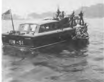
IUW-65, a harbor patrol boat, looking more like a pleasure boat than a Navy picket vessel, stops to investigate a small Vietnamese boat. The harbor patrol boat's large size allowed the HPE to carry out longer patrols and gave it the ability to carry heavier weapons such as the twin .50 caliber machine guns mounted amidship. The crew are armed with shotguns, M-16s, and side arms. (US Navy)
