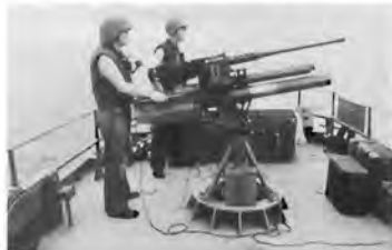
The combination mortar/machine gun was mounted on Swift boats and 82 foot Coast Guard cutters. Because of the way the weapons were sited it was not possible to fire both at the same time. The oversized helmet worn by the gunner contains communication gear which is connected to the bridge via the cord running across the deck, allowing the boat commander to direct the gun fire. (US Navy via Bell)
