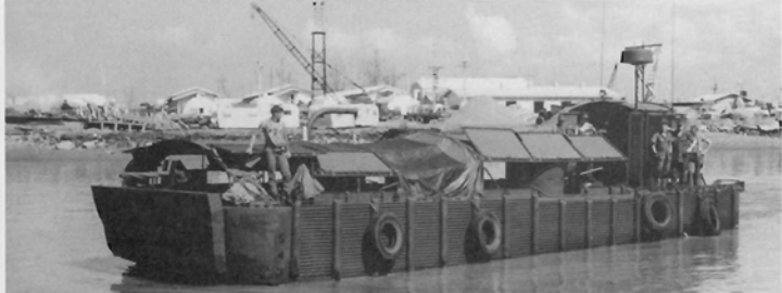
This landing craft has been converted to a river minesweeper (MSM) for use along the waterways in Vietnam. A number of these were employed along the river leading to Saigon and in I Corps. This particular vessel is coming into Nha Be after a mission on the Long Tau. (US Navy)
