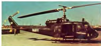
(Above) This UH-1M Huey of HAL-3 sits on the runway at Binh Thuy just prior to the squadron's stand down in January of 1972. The UH-1M was an upgraded version of the UH-1C. (Mesko)
