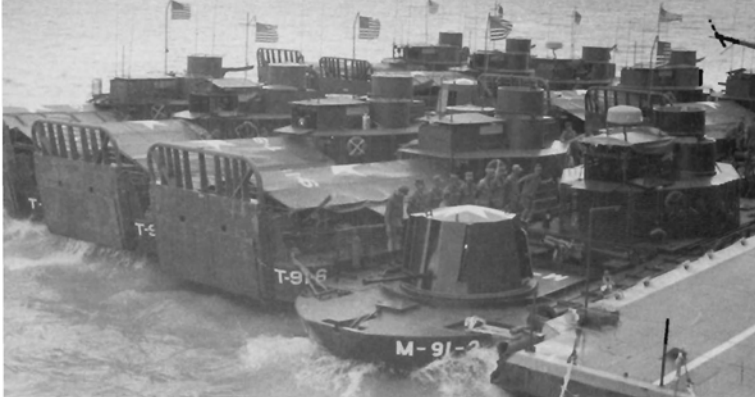
These ATCs and Monitors from RAD 91 sit along side an Ammi pontoon prior to an assault into the Delta. Even in the relatively confined waters of the Delta riverways the water could get choppy as is evident from the spray raised by the bows of the moored boats. (US Navy)
