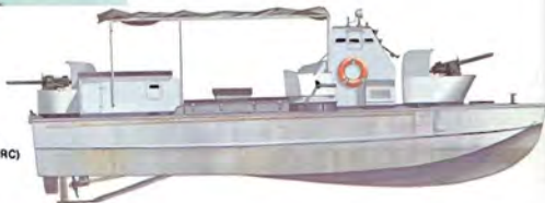
(Above) Another type of motorized junk with a more upswept bow also carries a protective eye on its bow, but instead of the standard .30 caliber machine gun on the bow a more potent .50 caliber machinegun has been mounted with a protective shield. (Chanowath)
