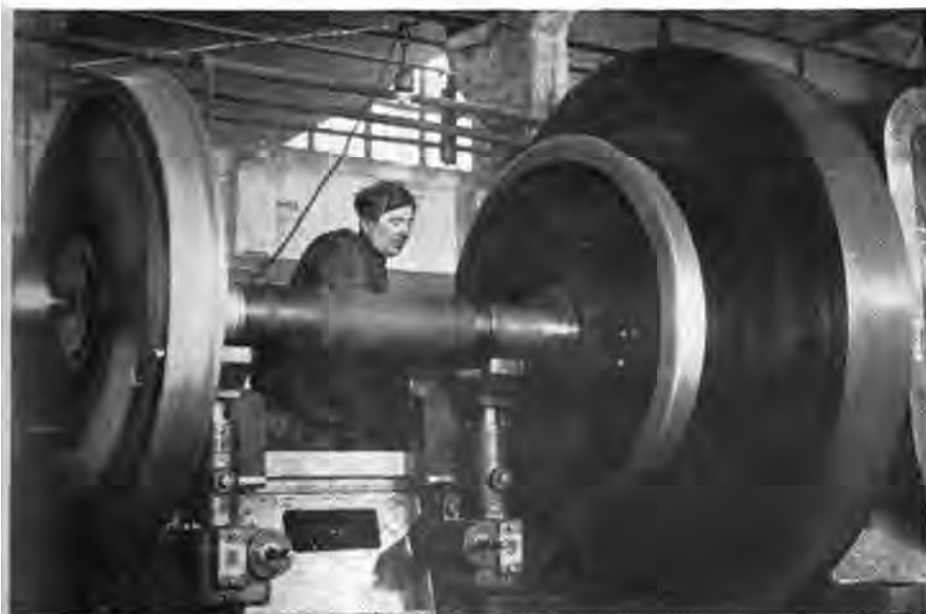
Grinding locomotive wheels in a new machine engineering plant built in Krasnoyarsk, Siberia. The workers kept the transport system operating throughout the war
