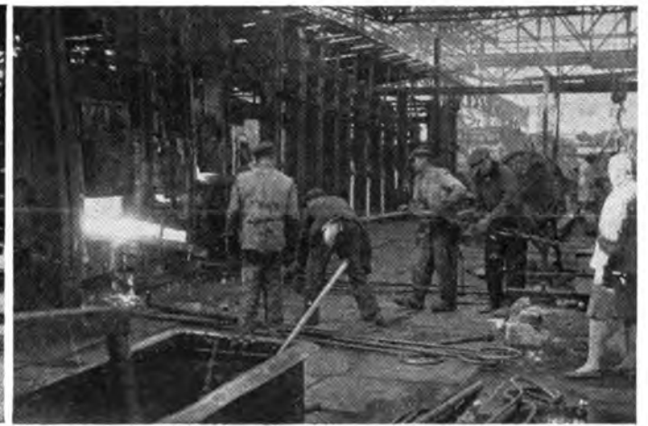
At the Krasny Oktyabr iron and steel production works the restored shops are now in full swing. Left, pouring steel from an open-hearth furnace, one of the seven which have resumed operation. On the right, workers remove a steel ingot
