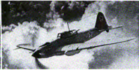
The armored IL-2 "Stormovik" attack plane, designed by Hero of Socialist Labor S. V. Ilyushin
