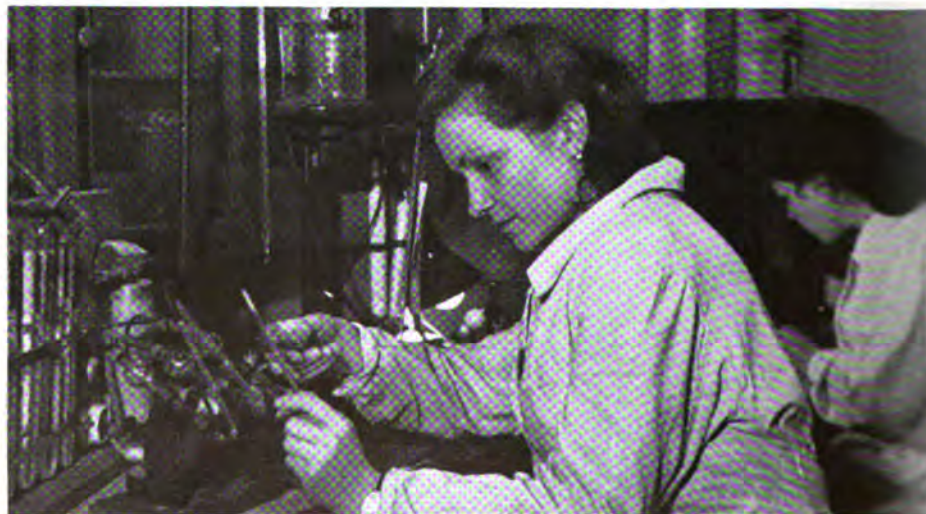
Analysis of the air in various parts of the plant—testing for carbon dioxide
