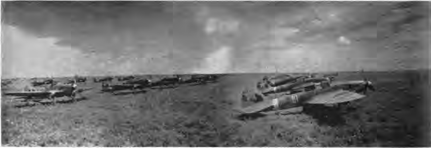
"BLACK DEATH"—the Germans' name for the Soviet IL-2 Stormoviks, designed by S. Ilyushin. Above, a group of these low-flying, heavily-armored planes are about to take off
