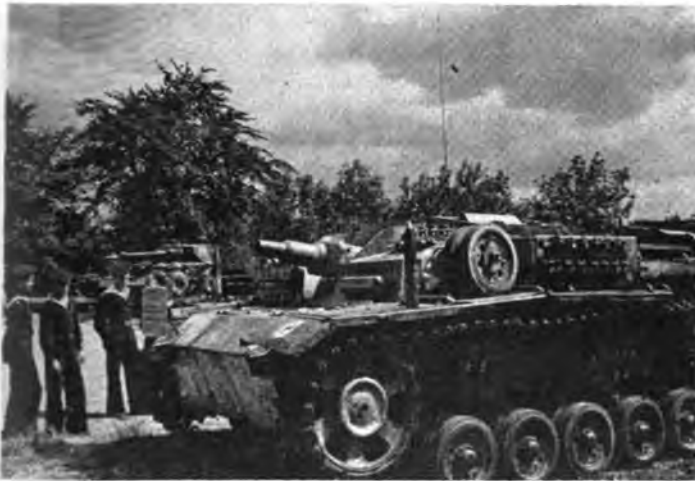
The 75-mm. self-propelled gun—the "Artsturm"
