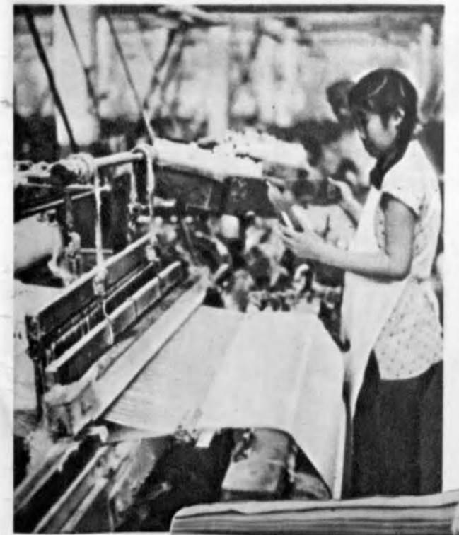
**WEAVING**—a reed separates the warp threads and beats up the weft threads, weaving the yarn into cloth
