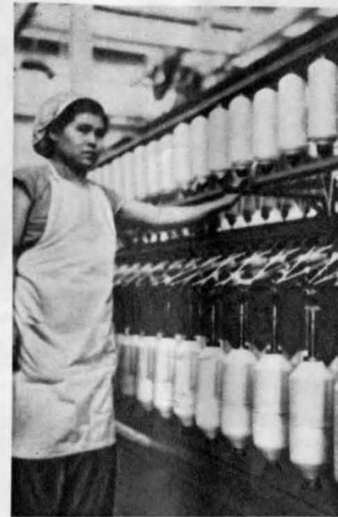
**COARSE SPINNING**—the rovings are set on an intermediate frame and spun into coarse yarn
