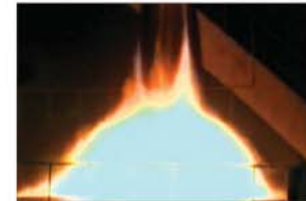
Success in a test that simulates the nose cone tip's re-entry into the earth's atmosphere
