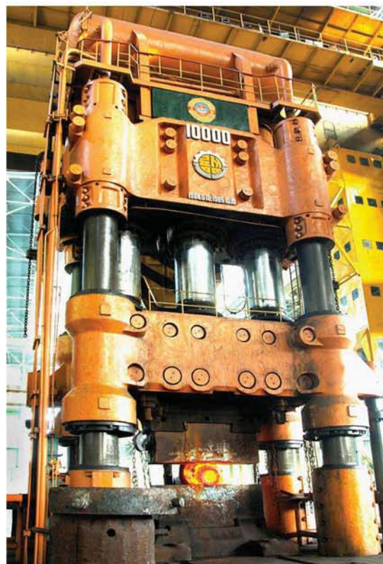
A 10 000-ton press equipped with CNC technology.
