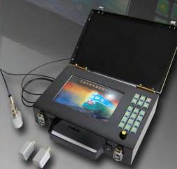
With a transmitter that can monitor the depths of over 5 000mm in the axle to detect cracks and a receiver that can amplify the signal up to 80 dB, it can continue detecting for over 8 hours through minimized power consumption as suited to its portable character.
