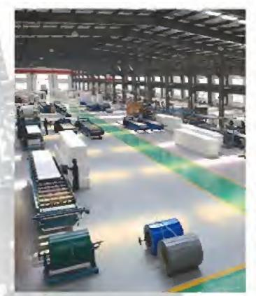
The factory has workshops for roofing plates, light-weight steel frames, plastic building materials and concrete blocks, which are operated on PLC flow line.
