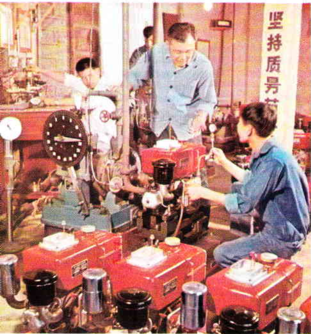
Inspecting diesel engines.
