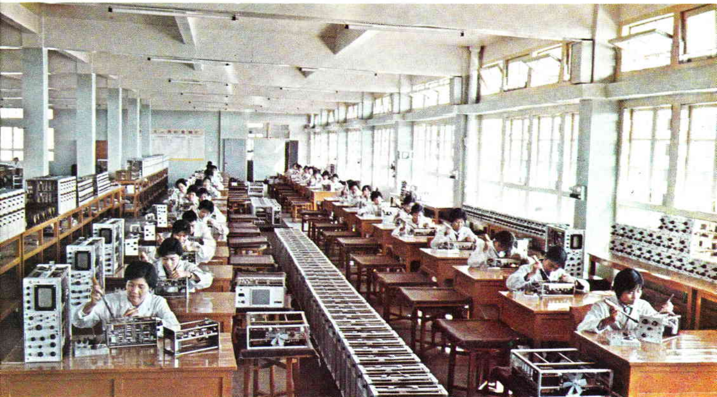
Ultrasonic flaw detectors being assembled in the Shantou Ultrasonic Instruments Factory.
