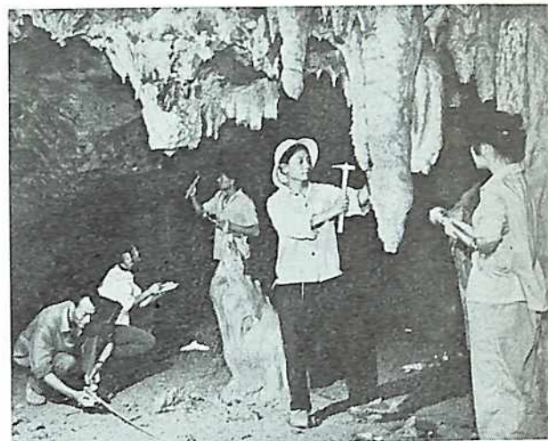
A Szechuan province hydrogeological team investigating an underground solution cavity in search of water sources for irrigation.
