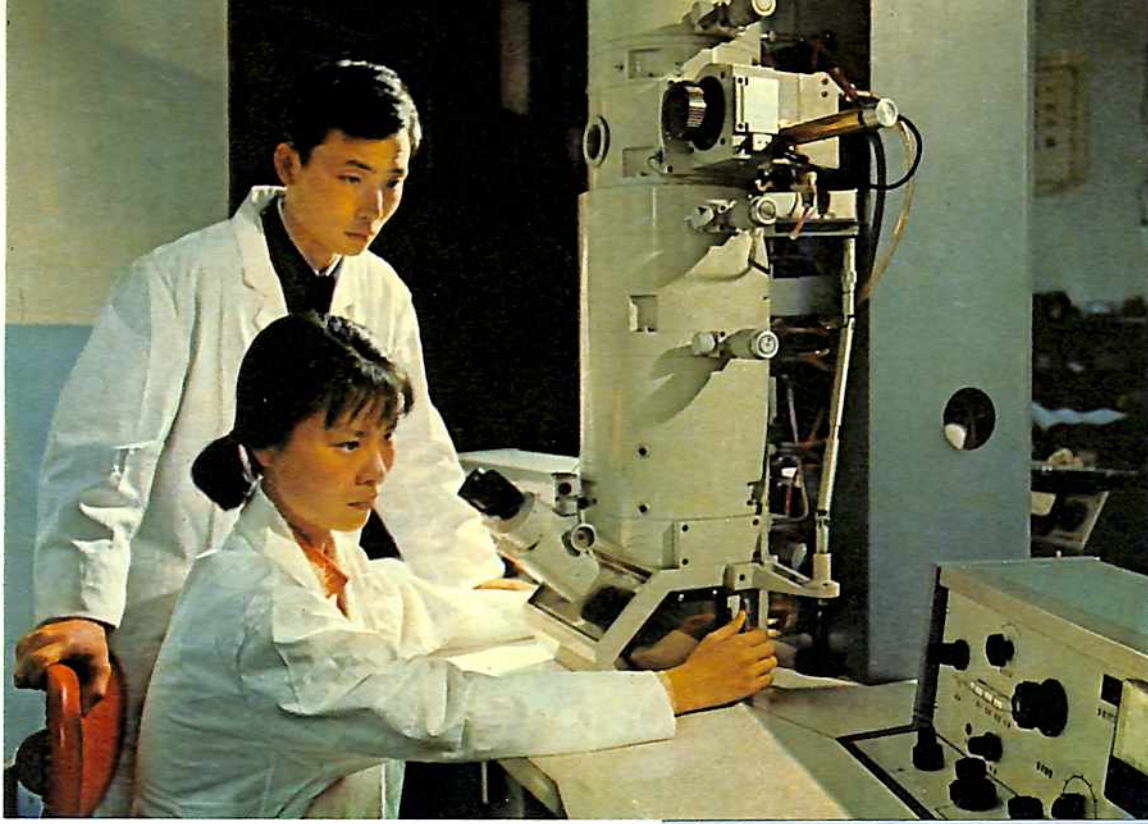
China's first 800,000-power electron microscope developed by the Shanghai Hsinyueh Instrument Factory.
