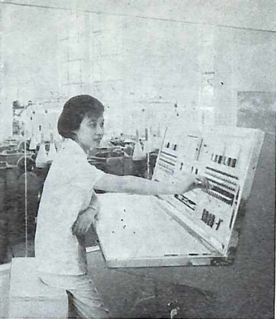
Shanghai's glove industry has used computers to control groups of glove-knitting machines, raising productivity 28-fold.
