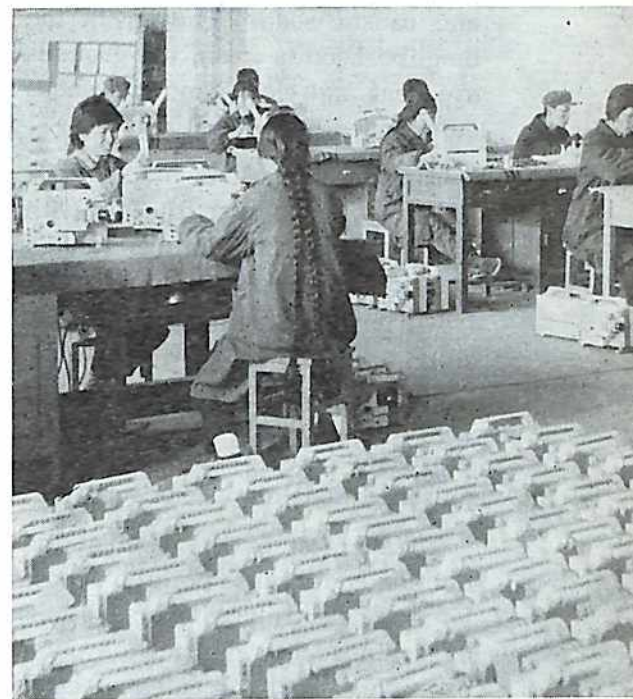
Workers at the Kansu Optical Instrument Plant assemble 8.75-mm. movie projectors.
