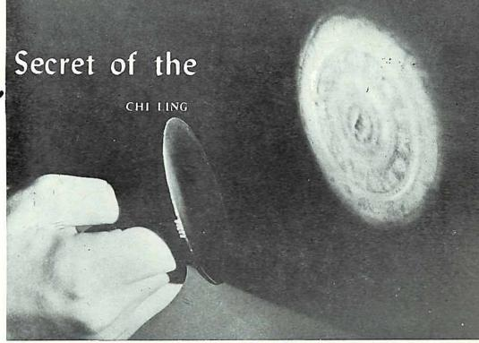
The smooth side of the mirror reflecting on the wall the designs and characters on the back.
