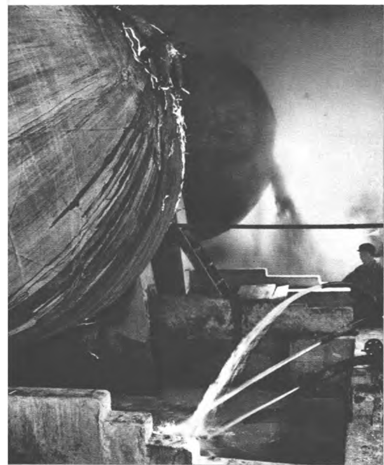
In a small-sized paper-making mill in Wuan County, Hopei Province, there are only over 100 workers and staff members. They were the first to use wheat-straw pulp in successfully trial-producing thin letterpress paper, thus making a contribution to the dissemination of the great Mao Tsetung Thought. Upper: Digester for preparation of wheat-straw pulp. Right: Thin letterpress paper produced by a locally-made paper machine.
